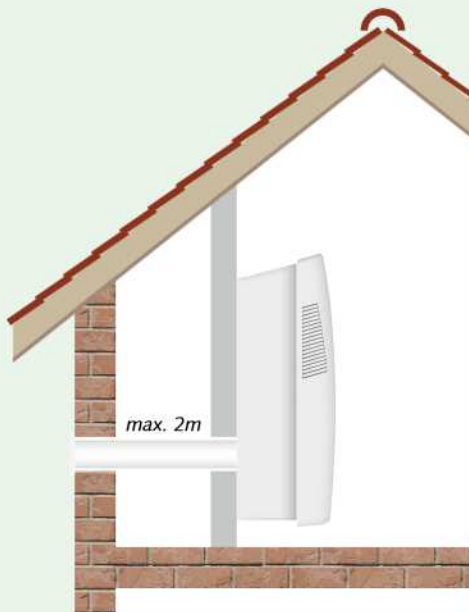
Flexible application possibilities due to the installation of an air channel
